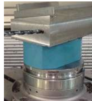
Special version for pallets on 5-axis machine
