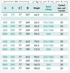
Other sizes and rated voltages on request. Larger chucking areas can be implemented by joining several blocks without gaps. Allocation to the correct control unit is based on the max. power consumption/magnet voltage.
